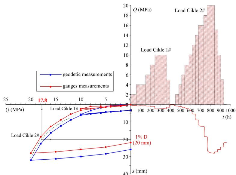
Figure 5. Results of a pile load test
