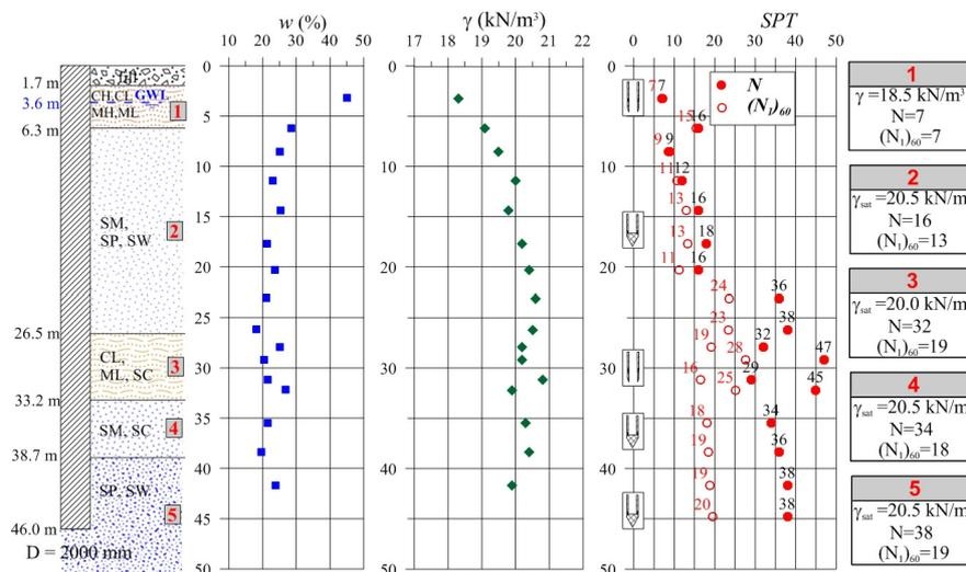
Figure 2. Physical-mechanical characteristics and accepted geotechnical terrain model
