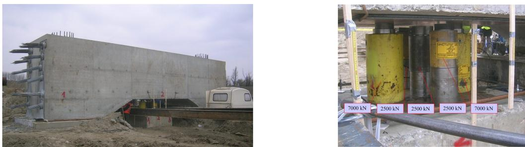
**Figure 4.** Display of the system for pile test load with locations of hydraulic presses
