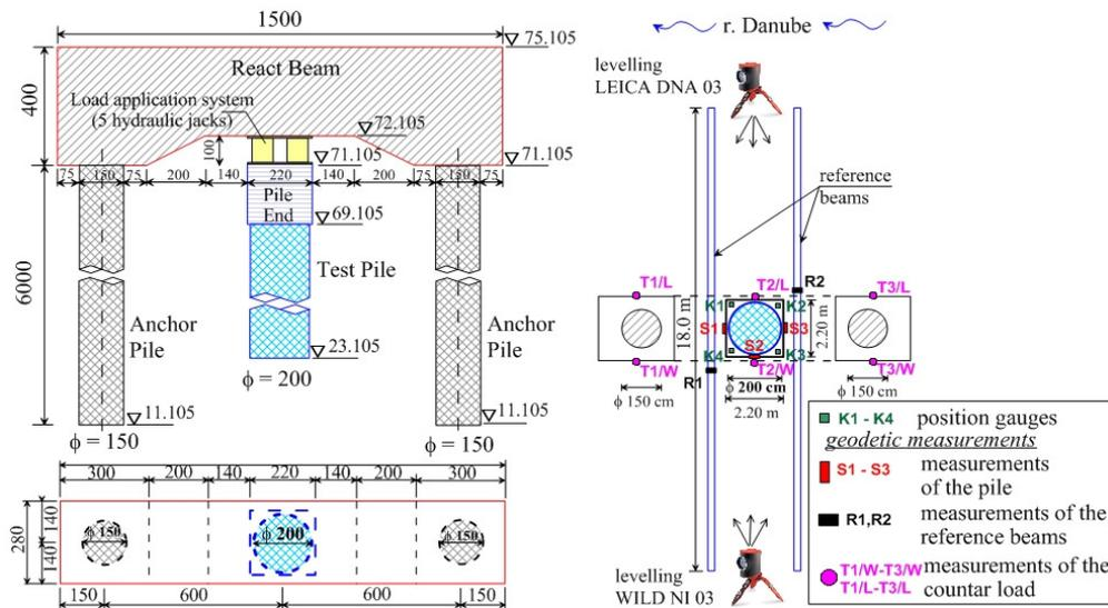
**Figure 3.** Static load test structure with location of gauges and points of geodetic observation
